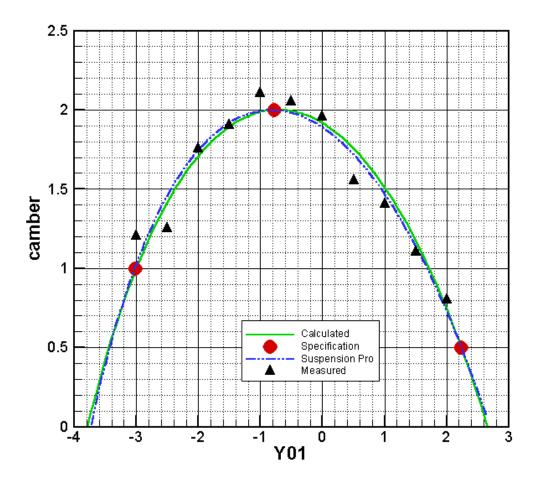
The triangles in the figure were measured on a TR3 with suspension that was stock except for springs which lowered the car about 0.3 to 0.4 inch. Camber measurements were made using a digital level or digital protractor.
