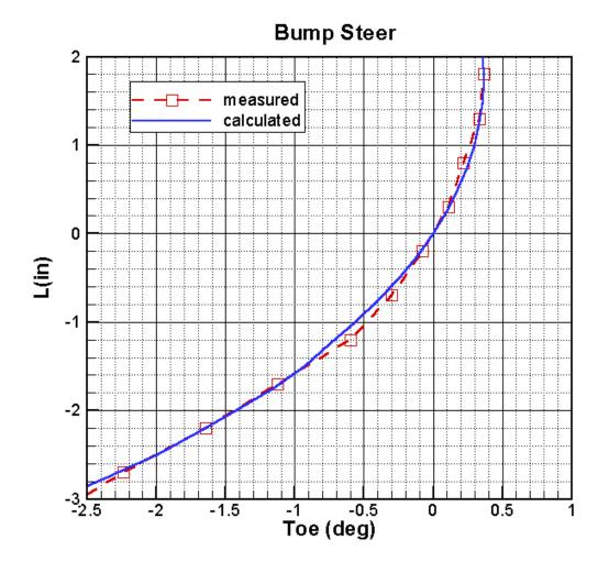
the observation that the car was unstable under hard braking. The software was then used to determine how to eliminate this problem. Bending the steering lever up 1/4 inch is sufficient to eliminate the bump steer problem. Lowering the car would also improve bump steer, because the toe variation is reduced in the bump direction.
